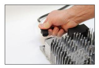
2. Reconnect the AC input while continuing to press and hold the Charger button.
