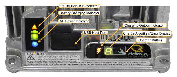
1. When you plug into AC power, the **AC Power Indicator** illuminates solid blue to indicate AC power is present.
