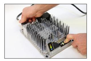
3. Continue to hold the **Charger** button until the **Error Display** illuminates amber and the **Battery Charging Indicator** is flashing green (wait maximum 22 seconds). Release the **Charger** button.
