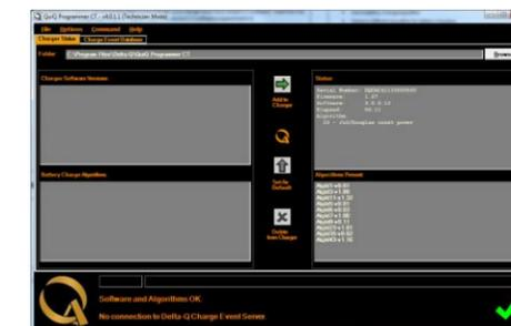
If the connection area displays **Status: No Connection**, then QuiQ Programmer is unable to communicate with your charger. This may be due to one of the following:
