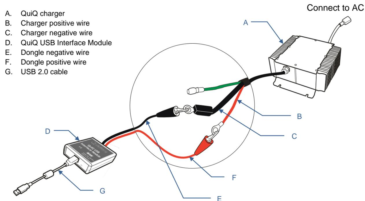
Figure 1. Wire connections for Programmer setup
