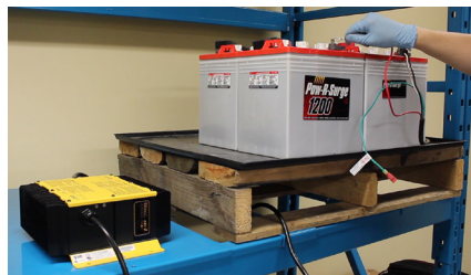
Figure 7: Touch the positive lead to the positive battery terminal for 3 seconds.
