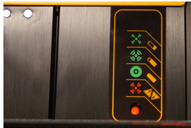
Figure 4: Red fault light blinking
