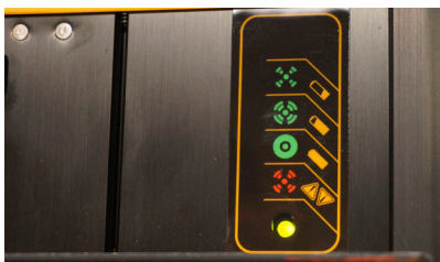
Figure 3: Default charge profile is displayed by the green flashing LED
